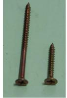
MULTI USE SCREWS BUGLE HEAD. NEEDLE POINT PHILLIPS DRIVE YELLOW ZINC FINISH FOR INTERNAL USE FOR GENERAL FIXING INTO TIMBER OR LIGHT GUAGE METAL WHERE A COUNTERSUNK HEAD IS REQUIRED 6 GUAGE & 7 GUAGE 20mm to 75mm AVAILABLE IN HANG PACKS, JARS, PAILS WITH HANDLE AND BOXES
